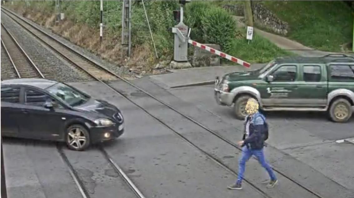
Vehicles crossing the level crossing in the middle of the process of closing semi-barriers
