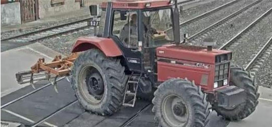
Obstacle not detected by the induction loop system
